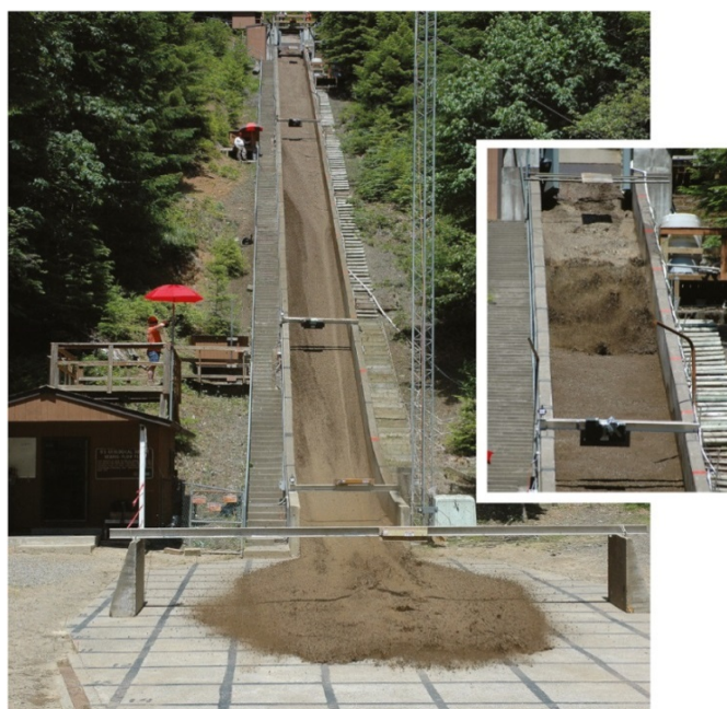
Figure 1.2. Photograph of the large-scale (95 m length) USGS debris flow flume used for debris flow experiments (From Iverson et al., 2011).
