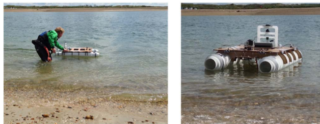
Fig. 1. A student retrieving the Pytheas unmanned boat after completing 3 return journeys crossing the 400-m wide open seawater between Southsea and Hayling Island within 10-m diameter of the predefined GPS coordinates (waypoints) based on the online map service by Google®.
