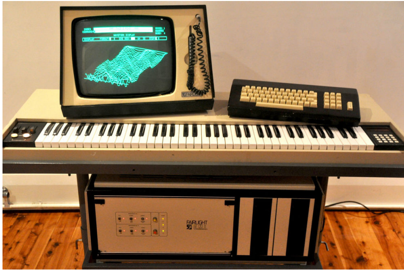
Fig. 10. The Fairlight CMI (Computer Musical Instrument) Mk. 1 (1978)
