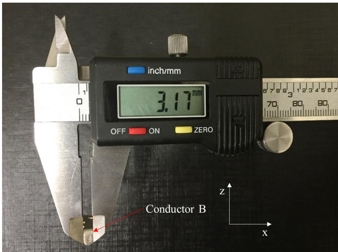
Figure 4.21. Length measurement between particular characteristics of the Conductor B using a standard micro-meter
