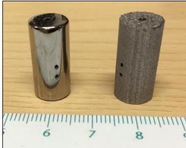
Figure 11: Photograph of Ti-6Al-4V implant model manufactured via selective laser melting. As- fabricated part (right) and polished part (left).
