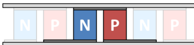
Figure 9. Schematic diagram of a thermoelectric module, with a pair highlighted. The pairs are connected electrically in series through metallic contacts (dark grey) and thermally in parallel through ceramic plates (light grey). This configuration allows for the maintenance of a temperature differential from one ceramic plate to the other through the thermoelectric material.
