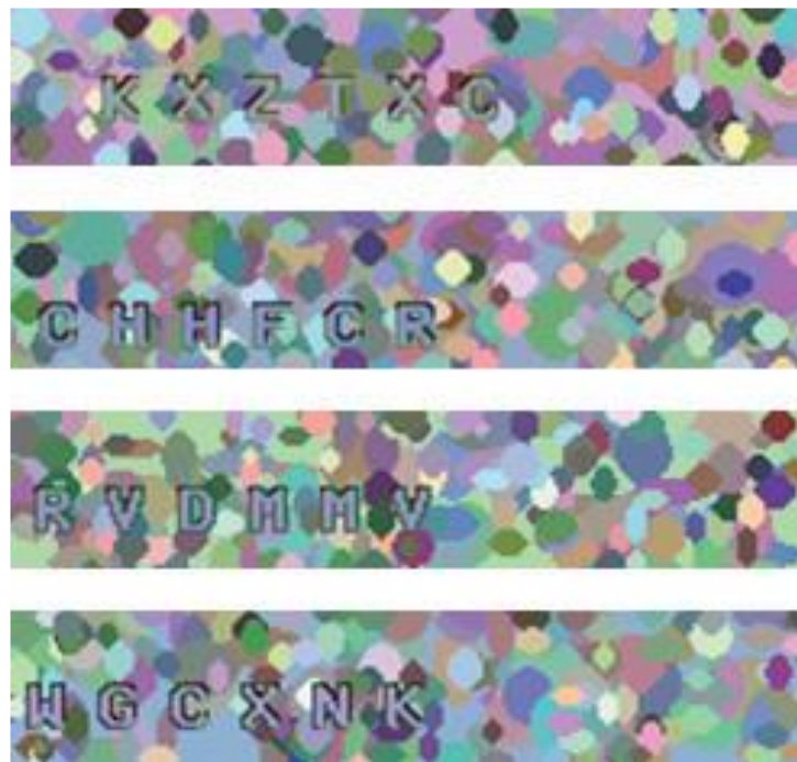
Figure 2.25: Example of the BotBlock CAPTCHA. Using the same colour for the test and background noise would make the CAPTCHA difficult to recognise for the human users.
