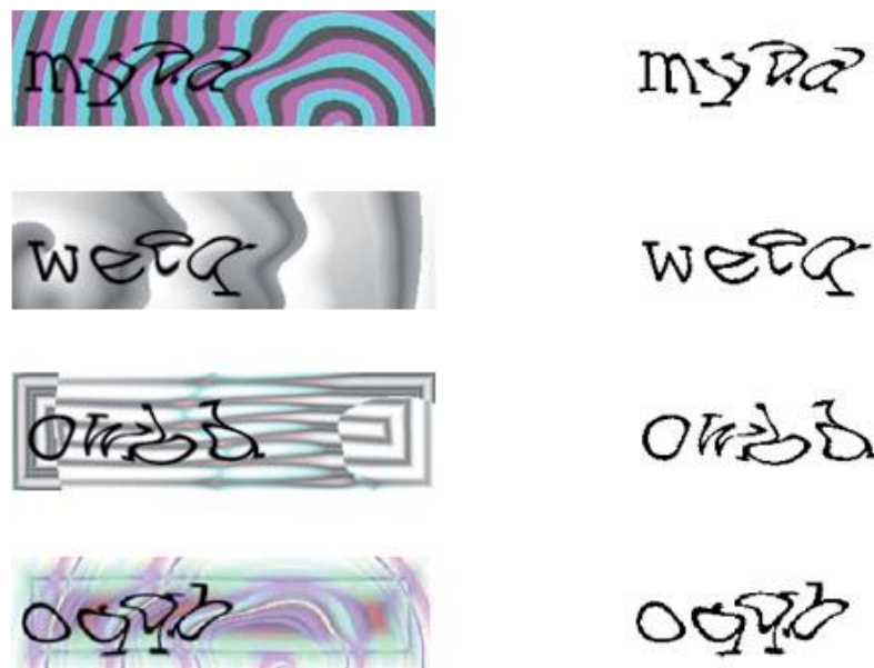
Figure 2.24: Using the colour matching algorithm to break the Gimpy CAPTCHA challenge. As the examples showing, using distinct colour for the text and background noise would make it easy for the OCR to filter the colours.
