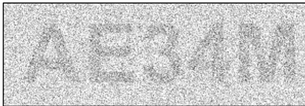
Figure 4.30: Final integrated output result from superimposing 10 CAPTCHA frames shown as an 8-bit/pixel greyscale image. A string of 'AE34M' can be clearly retrieved by OCR recognition software.
