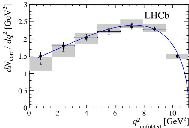
Figure 5: Comparison between the fit to the seven experimental data points using either the Lattice QCD calculation of Ref. [19], shown as grey points with a shaded area corresponding to the binned  $1\sigma$  theory uncertainty, or a single form factor fit in the  $z$ -expansion, shown as the solid blue curve. The data points, modulo a scale factor, are shown as black points with error bars.
