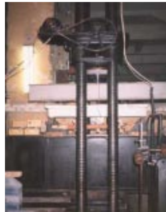
Fig. 2 Test setup of a typical test beam
