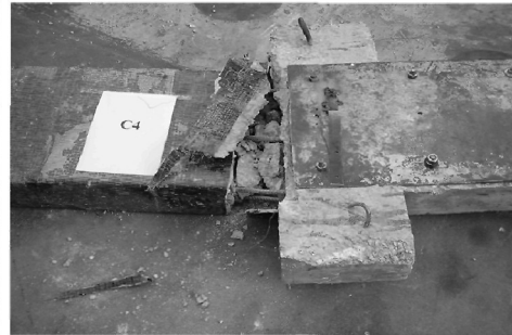
Figure 11 Failure of Specimen C4
