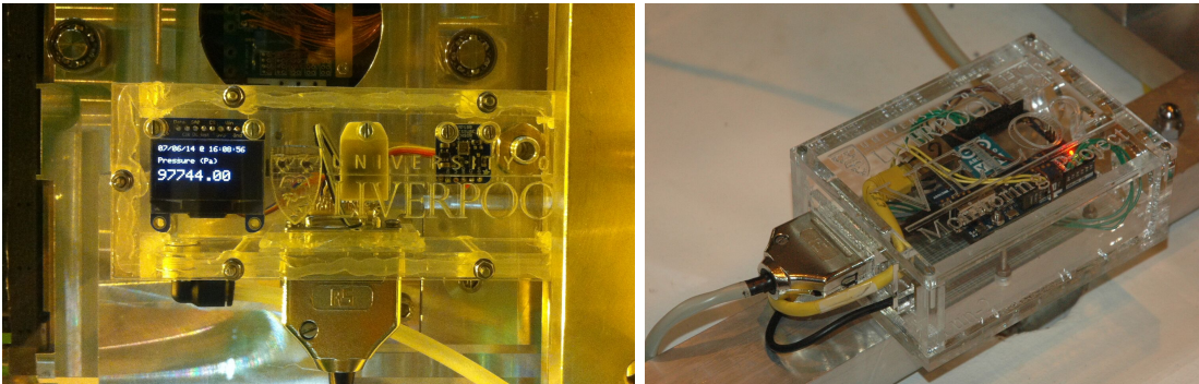
Figure 3.22: Left: upper half of the monitoring device containing the atmospheric sensors and the LCD currently displaying the pressure reading; right: lower half of the monitoring device containing the Arduino micro-controller board, the accelerometer and the power and network connections. The two are connected via a custom-made cable.
