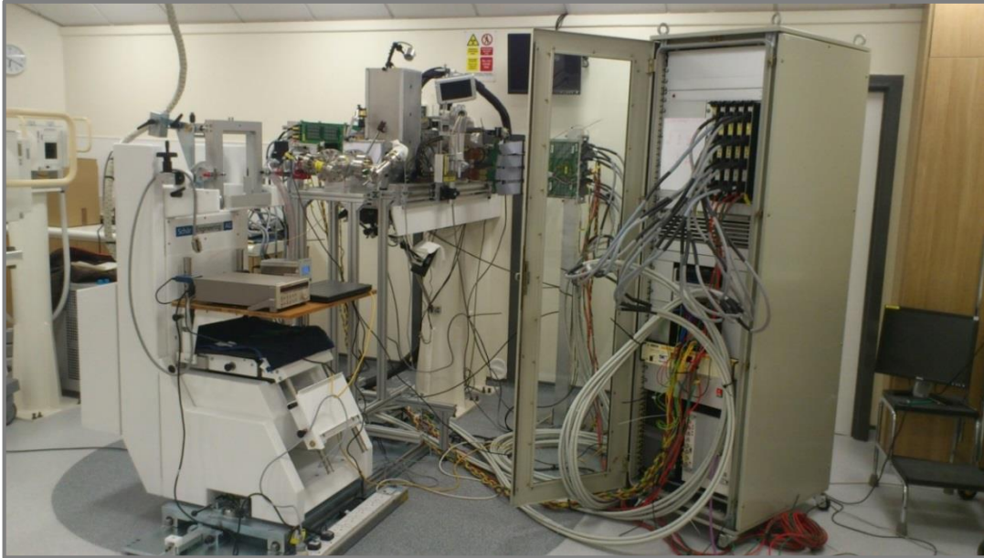
Figure 65: Overview of the non-invasive beam monitor test assembly at CCC: the stand hosting the VELO modules is visible behind the treatment box, a rack hosting the electronics on the right integrating TELL1 cards and their dedicated cooling, high and low voltage power supplies, DAQ computer and communication network. The FC vessel can be seen at the end of the treatment line in the top left quarter of the image.
