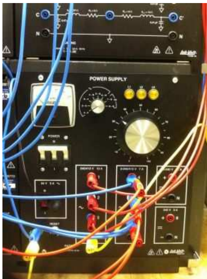
Figure 8.3: 3 phase power supply
