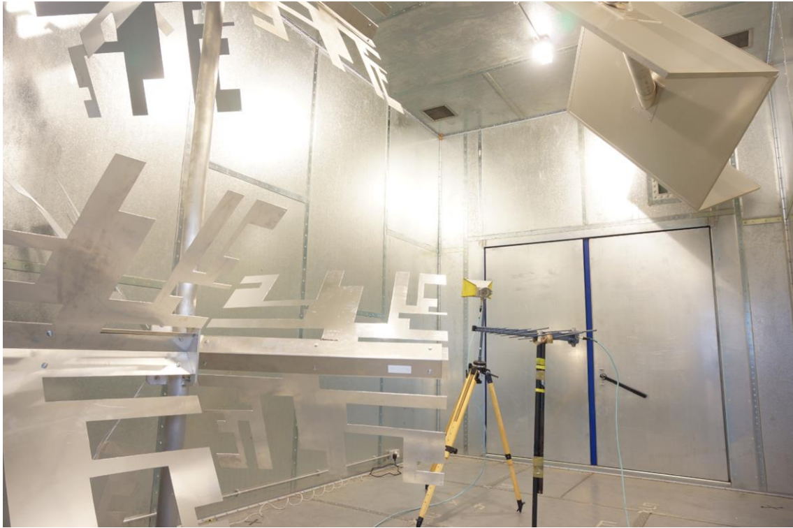
Figure 1.4 Photograph of a typical measurement setup in the RC at the University of Liverpool.
