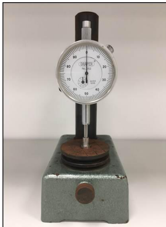
Figure 3.2: Dial thickness gauge used to measure the thickness of P&K hydrogels.
