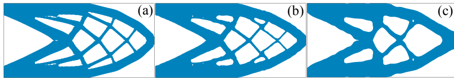
Figure 10: Cantilever 2:1 compliance solutions, with cutting surface discretizations: a) 32 \times 16 , b) 16 \times 8 , and c) 8 \times 4 elements.
