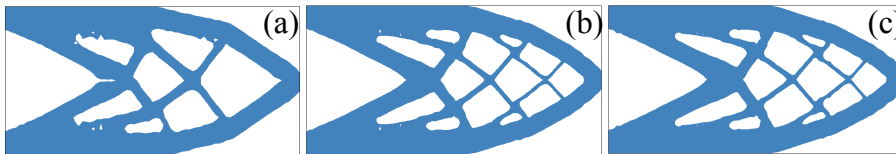
Figure 7: Mesh dependency. Cantilever 2:1 solutions using a cutting surface mesh of 16 \times 8 elements and an analysis mesh of: a) 80 \times 40 , b) 160 \times 80 and c) 320 \times 160 elements.
