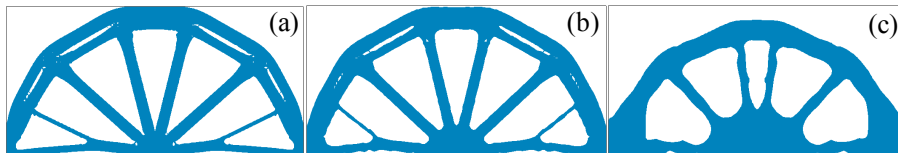
Figure 12: Simply supported Michell compliance solutions, with cutting surface discretizations: a) 32 \times 16 , b) 16 \times 8 , and c) 8 \times 4 elements.
