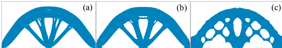
Figure 11: Clamped Michell compliance solutions, with cutting surface discretizations: a) 32 \times 16 , b) 16 \times 8 , and c) 8 \times 4 elements.
