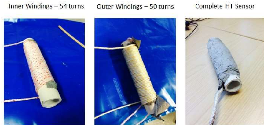
Figure 50: High temperature in-situ cylindrical EM sensor in different stages of construction, with only inner windings in the left most picture, with both inner and outer windings in place in the middle picture and coated in silica outer in the right most picture.
