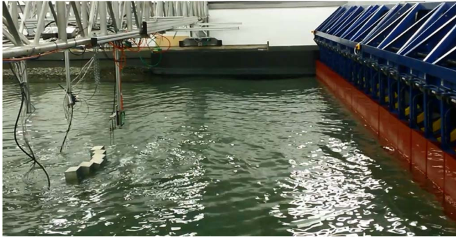
Fig. 3. Photograph of the physical model, in its Modular Flap configuration, operating in the wave tank.
