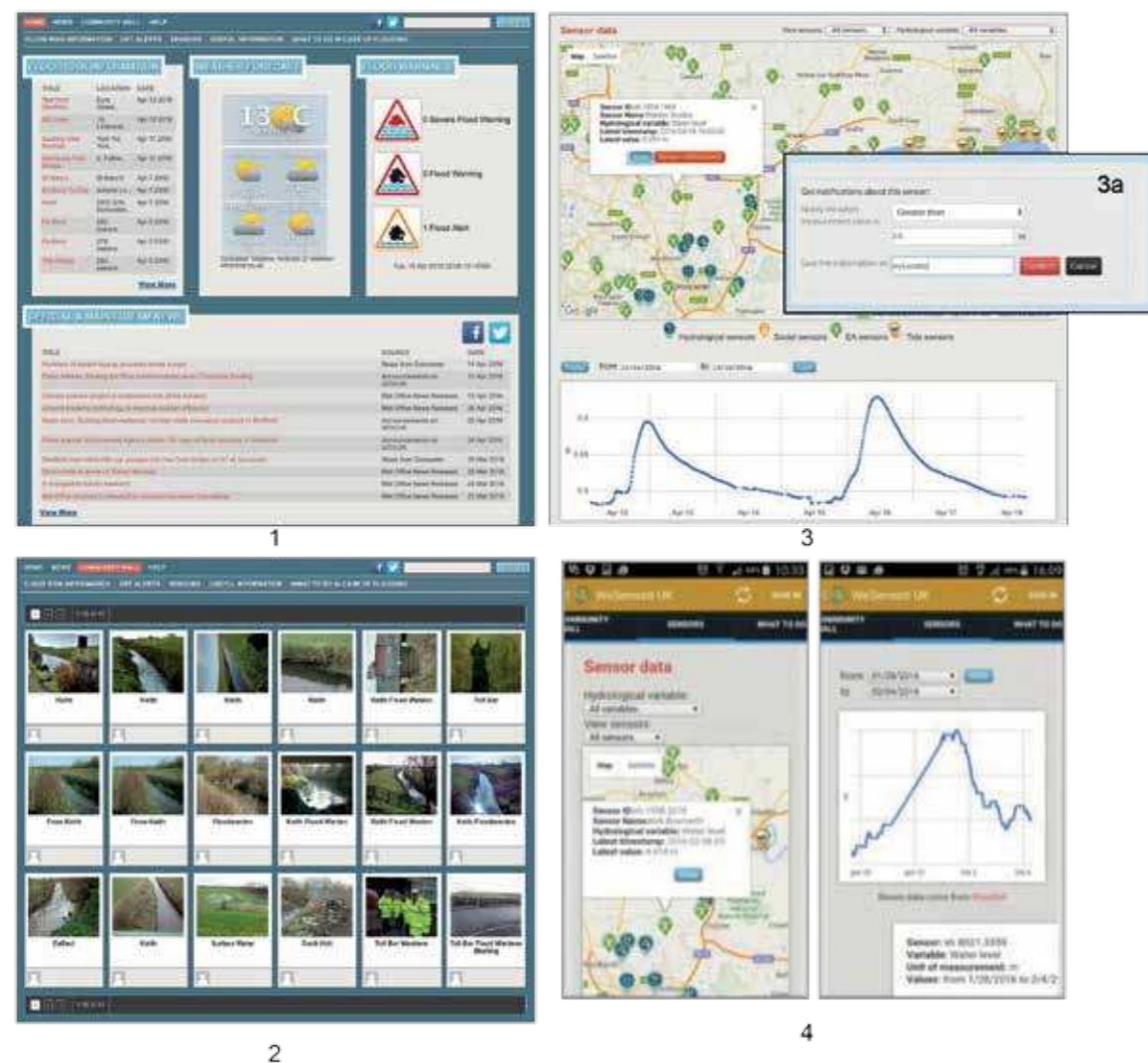
▲ Figure 5. Citizen tools for decision support. 1 - Home page for citizen portal, displaying essential information critical to the citizens' needs. 2 - Community wall displaying memories and images of historical events in the community. 3 - Sensor data visualisations and sensor notification subscriptions (3a). 4 - Citizen application providing the same information, but in a mobile phone format.
