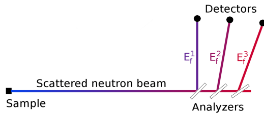
FIG. 1. A simplified sketch of the CAMEA concept. A vertical cut along one scattering angle is shown. Scattered neutrons with several different energies will be detected separately. Ideally all scattering angles should be covered continuously.
