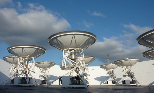
Figure 1. The SA telescope is located inside a metal enclosure with a metallic ground plane which acts as a reflector and also minimises radio frequency interference (RFI).
