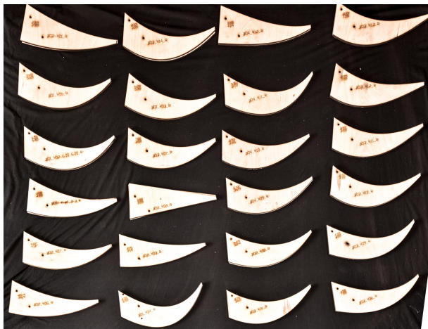
Fig. 2: (a) Morphology parameters are defined as curvatures at discrete points on the foot, and the foot shape is derived through integration of the curvature resulting in 2D foot shapes in a Height-Length domain. (b) Foot shape samples which were designed by the model-free design optimisation for improved locomotion speed in the robot.
