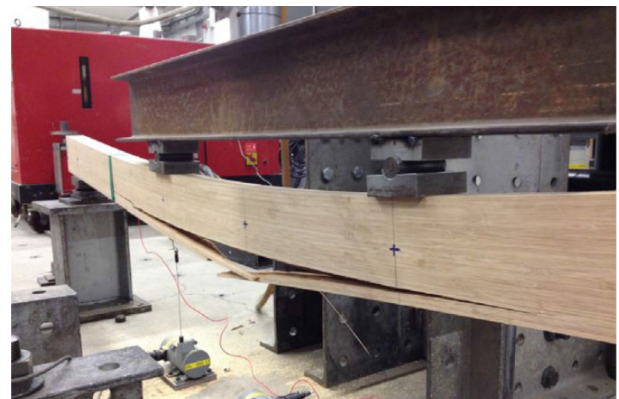
Fig. 2. Four-point bending apparatus used in the testing of all beams.
