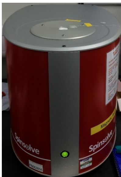
Figure 8.2: Benchtop 43 MHz spectrometer in which a 5 mm tube is lowered into the centre and secured using strips of adhesive tape. Dimensions (in cm): 58 \times 43 \times 40 .
