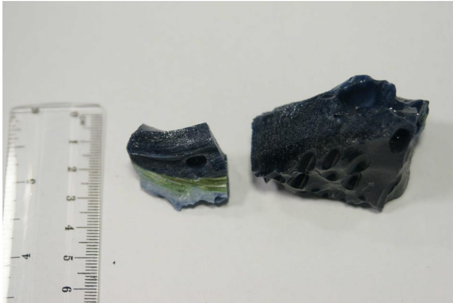
Figure 21: An image of one part of the wasteform as received.
