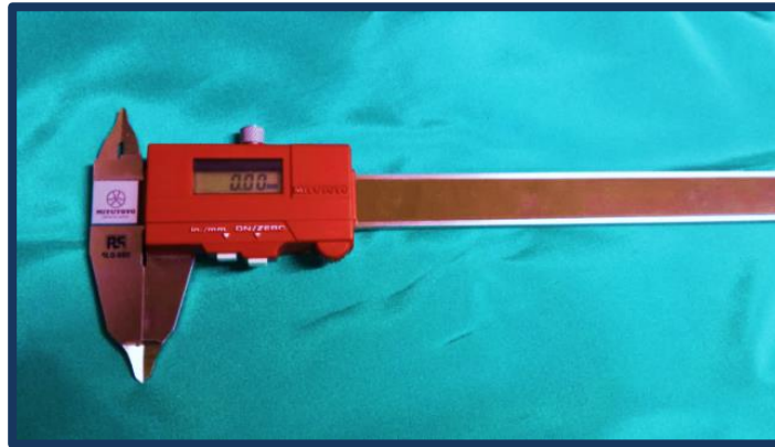
Figure 6.2 Photograph of the digital calliper used to measure specific features of the class II amalgam cavity for the upper second premolar
