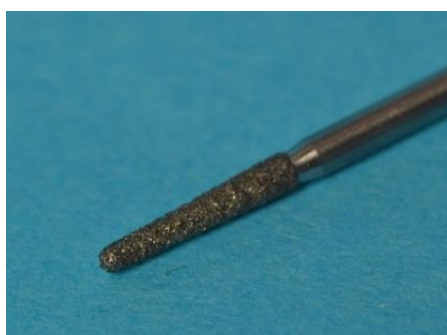
Figure 3.2 Picture of a tapered high-speed diamond with a rounded tip (Chamfer) bur
