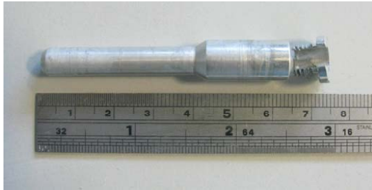
Figure 8. The mid height pore pressure transducer attachment used for 180,000% repeat test.
