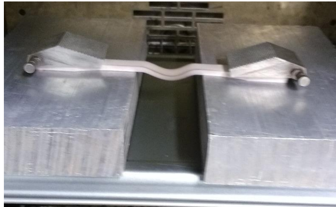
Figure 2. Photograph showing the sag which has occurred to a test coupon held at a temperature of 190°C
