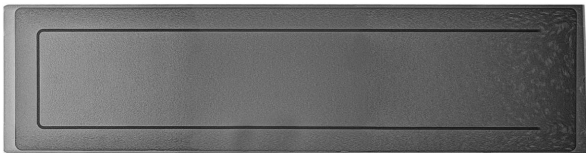
Figure 6.6. X-Ray scans of PP 20GF foamed plates with IQ Foam® and combined with Core Back technology.
