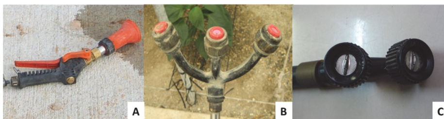
Figure 4 Types of spray output mounted in spray guns or lances: a) hollow cone variable flow nozzle; b) three fixed nozzles; c) double flat fan nozzle.
