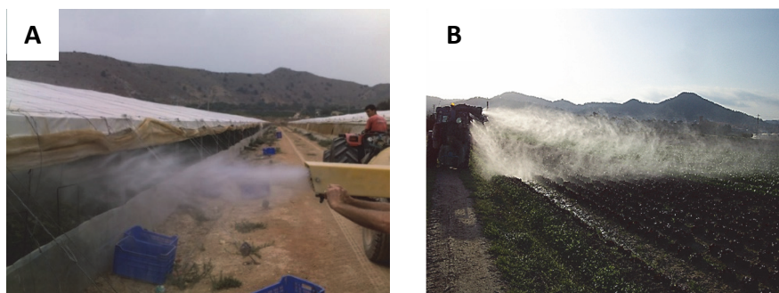
Figure 5 Cannon mist blower applications: A) spraying from outside of the greenhouse; B) spraying tall trees.
