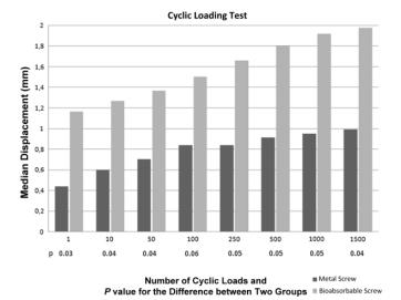
**Figure 3.** Loading-induced displacement (mean  $\pm$  SD) observed in the bioabsorbable and metal groups during the cyclic-loading test.
