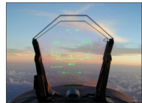
Image 2. Head-up display in an aircraft.
