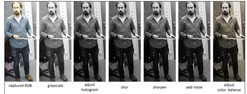
Image 6: Example of impact various steps of the SelfieWall image post-processing has on the image.
