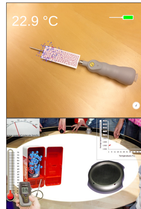
Image 1: Digital AR-thermometers—first and second version—developed to show the molecule movement’s speed in different temperatures
