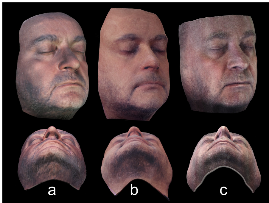
Figure 2 Pictures of 3D printed facial masks of the test person: a) DAVID, b) 123D, and c) Proface.
