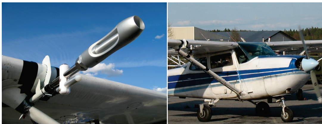
Fig. 1. Photographs of the inlet mounted on the right wing of the measurement aircraft.
