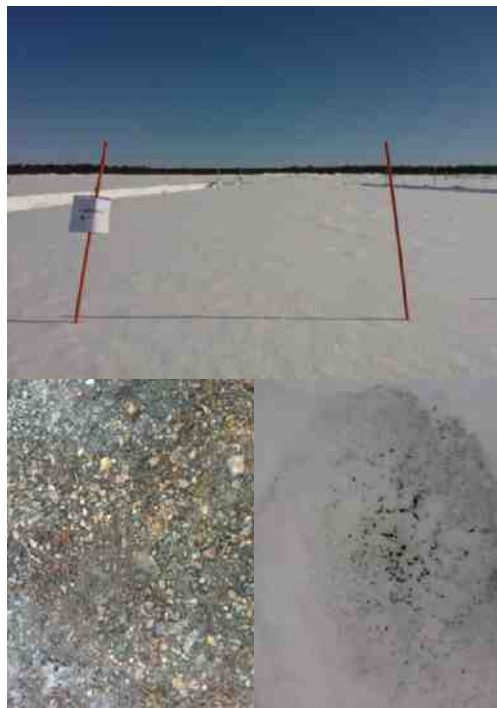
Figure 1. The SoS-2013 experiment. (a) Top: the flat and open experimental field with the seasonal snow pack; (b) bottom left: the ground under the snow, i.e. a natural gravel surface, not covered by concrete or asphalt, offered a uniform surface for the snow cover; (c) bottom right: previously added impurities were visible on the surface of the melting snow, here volcanic sand.
