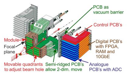
Figure 3.4.: Schematic view of the AGIPD megapixel detector [39]. From the analogue in-pixel storage the signal value is digitized by external 14-bit ADCs during readout. The detector implements storage cells for 352 images.
