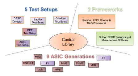
Figure 8.4.: **Design Goal for the Control Software.** A central library is needed to operate the variety of Test Setups and ASIC generations. Also two different software frameworks are used in which the control applications are written. The goal is to combine as much as possible within one library which implements central functionality for all setups and ASIC generations. The different compatibilities are indicated by the box and frame colors.
