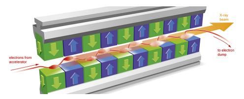
Figure 2.4.: Schematic view of an undulator. The alternating magnetic field forces the electron on an tight oscillating path which induces spontaneous synchrotron radiation [8].
