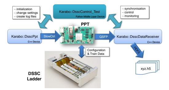
Figure 11.1.: **Overview of the DSSC Karabo devices.** The *Karabo::DsscControl\_Test* (KCRTL) device implements master control of the The *Karabo::DsscPpt* (KPPT) control device and the *Karabo::DsscDataReceiver* (KDR) device, which implements the data reception and pixel reordering. The KCRTL provides a simplified interface to initialize and control the other devices. Its main feature are automated parameter sweeps including generation of measurement log files.
