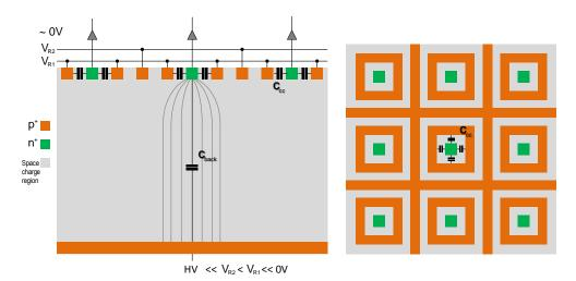
Figure 5.3.: Schema of a Mini Silicon Drift Diode [73]. The  $p^+$ -doped drift rings induce a good shielding from the neighboring pixels. The field lines are bended towards the small anode due to the applied ring voltages  $V_{R1}$  and  $V_{R2}$ .
