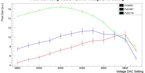
Pixel Gain using MSDD FE over Voltage DAC Setting
