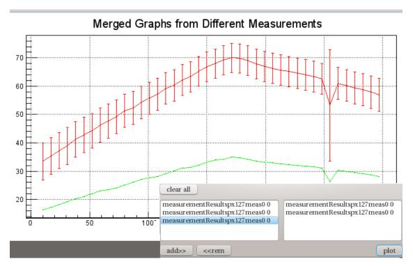
Figure E.10.: **The multiplot window and the output is shown.** The '*add*' and '*rem*' buttons can be used to change the graphs which are to be plotted in the output.
