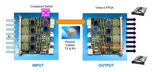
Figure 4.3.: Two XFEL Trainbuilder ATCA boards [45]. Due to their modular architecture, an ATCA board can either be configured as an INPUT or an OUTPUT. One board implements five Virtex-5 FPGAs. One master FPGA and four FPGAs, each of which are assigned to one Front End Unit. The connection between two boards is realized via a cross point switch and passive cables.
