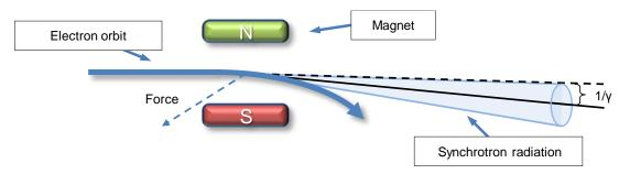
Figure 2.1.: Generation of electromagnetic radiation from a relativistic electron beam. Due to the Lorenz transformation, the emitted radiation is bundled in a narrow cone, tangential to the electron beam direction. The opening angle decreases with increasing energy  $\gamma$  of the electron beam. The power of the emitted synchrotron radiation scales with the forth power of the electron energy:  $P_{rad} \propto \gamma^4$ , where  $\gamma = E_e/m_e c^2$ .
