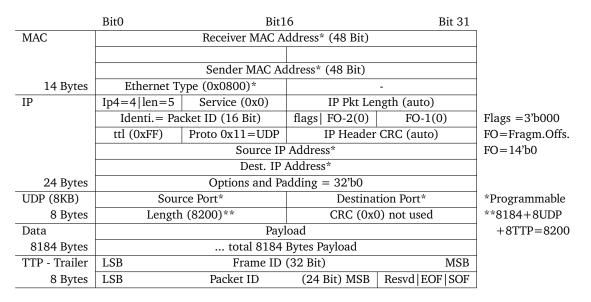
Table 7.2.: Ethernet Headers and TTP Trailer Bytes. Total 8236 Bytes per Ethernet packet, 54 Bytes overhead.
