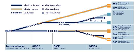
Figure 3.2.: The beamlines at EuXFEL [31]. Five tunnels will provide spots for 10 different experiments. At commissioning, only three tunnels will be equipped. Each undulator is assembled from 5-meter-long segments. The strength of the magnetic fields and the distance between the magnetic rails can be changed which allows to tune the generated wavelength.
