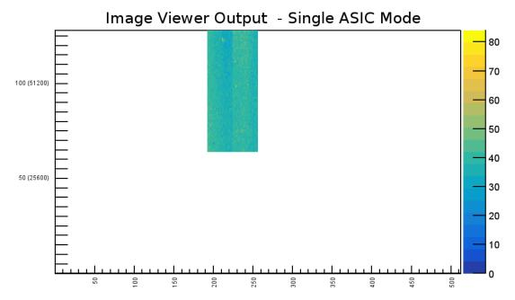
Figure E.9.: Image Viewer Output. Using the *Image Viewer* it is possible to generate images in Ladder format or single ASIC format. The current image shows a Ladder format image of a single ASIC measurement (ASIC 11).
