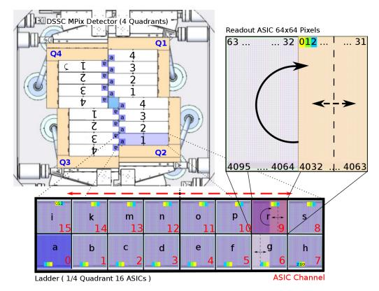
Figure A.1.: The numbering scheme of the Quadrants, Modules and ASICs of the megapixel DSSC detector.
