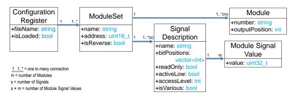
Figure 9.3.: Logical structure of the configuration register representation. For m modules and s signals,  $m \times s$  module signal values have to be stored. The structure is implemented by the *ConfigReg* class and allows to represent all kinds of configuration registers in the DSSC detector.
