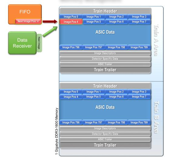
Figure 7.5.: DDR3 Memory Management. The 1 GB DDR3 memory on the PPT is divided into two Train Data blocks, which are filled alternately. The ASIC data region is subdivided into the image areas, which seamlessly store the image data. Due to the pixel word size of 2 Bytes, the addresses computation of the single image regions is fairly simplified.
