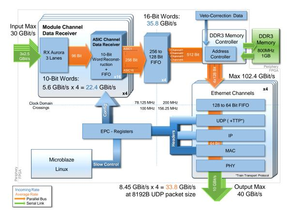
Figure 7.3.: **The PPT Data Path.** The data streams of four Aurora channels from the IOBs is received and the pixel words are re-constructed. In the DDR3 memory the Train Data is generated before it is packed into standard UDP Ethernet packets and transferred via the four 10 Gigabit-Ethernet links. Each module channel can be activated individually. The image re-ordering is implemented in the DDR3 address generator while the images are written to the memory.
