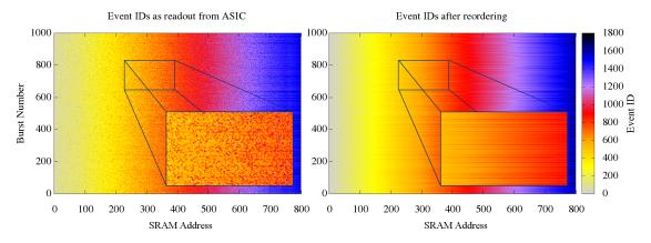
Figure 7.8.: Left: Veto Scrambled Image IDs as readout from the ASICs. Blue dots in red indicate SRAM addresses which have been vetoed twice, in orange even three times. Right: Image IDs after sorting.
