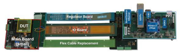
Figure 5.14.: **Image of the PPT Test Setup.** All basic components of the final Ladder are included: the PPT, one IOB, one PRB, one readout ASIC and the Main Board from the ASIC Test System.
