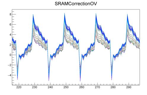
Figure E.5.: Mean SRAM value of 300 images (iterations) of 64 pixels from one measurement. The amplitude, frequency and shape of the systematic effect can clearly be seen in all selected pixels.
