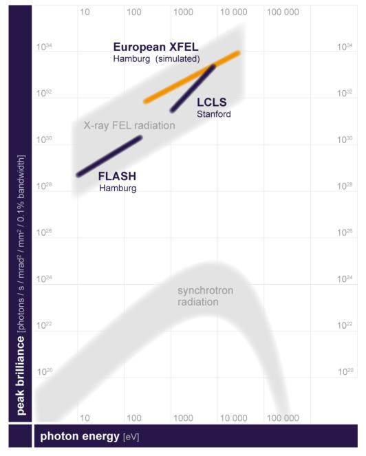
Figure 2.3.: The peak brilliance of free-electron lasers compared to synchrotrons [7]. FELs exceed the brilliance of the 3rd generation synchrotron radiation sources by up to ten orders of magnitude.
