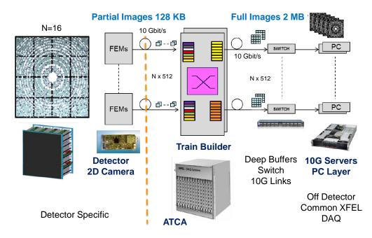
Figure 4.4.: **XFEL DAQ Environment [45].** One Trainbuilder collects all data from one megapixel detector via 16 10GE links. The Trainbuilder implements buffers and combines the data train wise, in order to transfer all data of one pulse train to the same receiver of the PC Layer.
