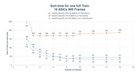
Figure 9.7.: Benchmark of the *Software Data Receiver*. The benchmark has been executed on three different machines for multiple number of sort-threads.
