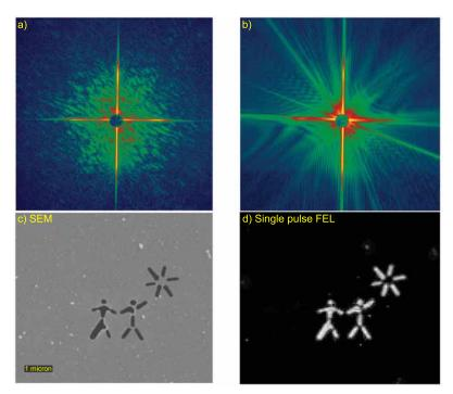
Figure 2.7.: Diffraction before destruction prove of principle at FLASH [31]. c) Ground truth, before the sample has been destroyed. The ground truth has been acquired using a scanning electron microscope (SEM). a) Diffraction pattern of a single soft X-ray shot, before destruction. b) Diffraction pattern after destruction. The pattern suggests massive changes of the sample. d) Reconstructed pattern from a), the spacial resolution has been estimated to 62 nm.
