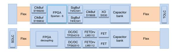
Figure 5.10.: Building blocks of the IOB [83]. Top and bottom view.
