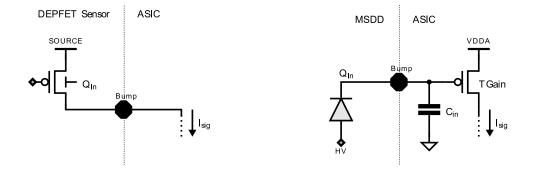
Figure 5.6.: Schematic drawing of the sensor readout concepts [73]. The front-end in the readout ASIC is designed to evaluate the current signal from the DEPFET (left). For the adopted MSDD of the F1 ASIC (right), the charge signal is translated to a current signal using a high gain transistor *TGain*.
