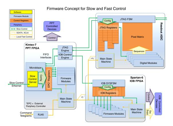
Figure 6.2.: Overview about the firmware concept for slow and fast control. The system is controlled and configured via the Slow Control Server running on the PPT. System synchronization is initiated from the main state machine on the PPT, which generates the fast control signals to synchronize the IOB and the readout ASICs. During image acquisition all peripheral devices are controlled from the main state machines on the respective devices. Only one of four IOBs is shown.
