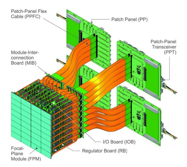
Figure 5.8.: Layout of the DSSC detector. (Courtesy of K. Hansen, DESY)
