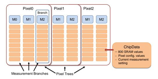
Figure 10.2.: Scheme of the root file storage structure. All measurements of the same pixel are stored in the same root tree as separate branch. The branch elements store all data for all iterations and settings linearly in the branch.
