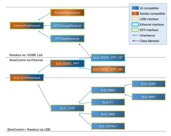
Figure 9.2.: Inheritance diagram of the DSSC control and readout software. The class provides pure virtual functions, which provide the access to readout and control functionality without implementation. The hardware specific implementation is realized in the derived classes.
