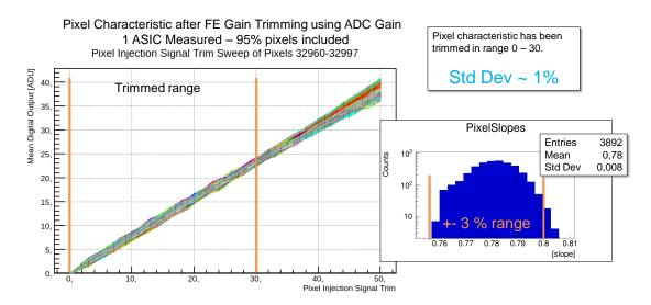
Figure 10.11.: Pixel gain distribution after trimming. One ASIC has been trimmed, and evaluated using the Pixel Injection. 95% of pixels could be trimmed in the target region  $\pm 2\%$ .
