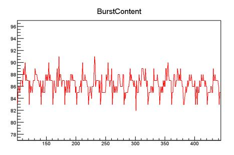
Figure E.4.: Image data from pixel 1024. The measured pixel was configured to the highest front-end and ADC gain in order to express the systematic effect as strong as possible. The amplitude is about 8 ADU.
