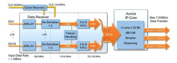
Figure 7.2.: **The IOB data path.** Recovery of the serial data from the 16 ASIC channels is realized by 16 data receiver modules. Each module implements a 1-to-3 'ISERDES' deserializer which implements distinct logic cells in the FPGA I/O region. The 3-bit stream is filled into a 3-to-6 FIFO that provides a buffer and implements the clock domain crossing. To compensate for misalignment of the incoming data to the data clock, each channel provides a distinct delay module.
