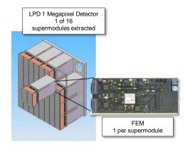
Figure 3.5.: Schematic view of the LPD 1M Pix detector [40].
