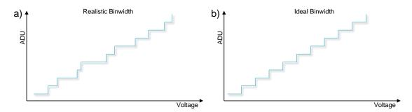
Figure 10.10.: **Realistic and ideal ADC characteristisc.** In a real ADC, the bin width varies. In the pixel ADC, a wide bin is normally followed by a thin bin.
