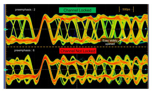
Figure 8.1.: Oscilloscope measurements of the signal quality. The signals have been measured at the input of the Aurora channel on the PPT. Tow different settings are shown. Best results have been achieved with swing = 10 and preemphasis = 2.
