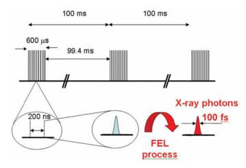
Figure 3.3.: Pulse scheme delivered by the EuXFEL [31]. The maximum pulse repetition rate is 4.5 MHz. The 99.4 ms pause is used for cooling and readout of the detectors.
