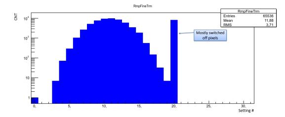
Figure 10.8.: Distribution of the resulting ADC gain setting in the Ladder. Start setting was 20. 16 of 64 (1/4) settings are assigned to compensate the pixel to pixel variations.
