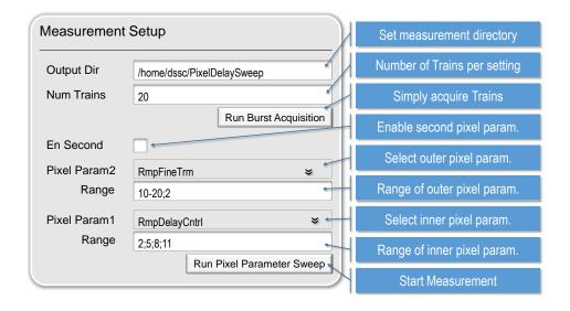
Figure 11.6.: Simplified view of the measurement control provided by the Karabo::DsscControl\_Test device. Two different measurement types can bee triggered. A very simple acquisition which just stores the specified number of trains and a more complex measurement which allows to step through two independent parameters of the pixel register.
