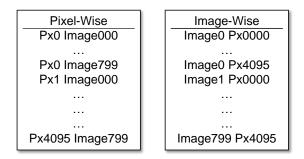
Figure 9.6.: **Pixel reordering modes.** Pixel wise is best for storing the data of pixel parameter measurements. Image wise is best for image visualization.
