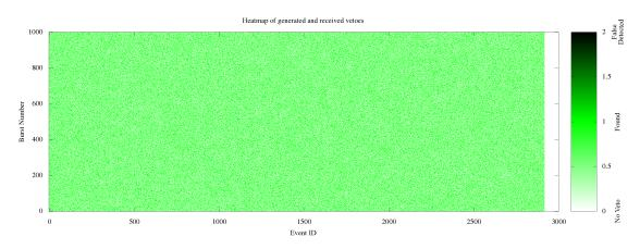
Figure 7.7.: Comparison of vetoed events and correctly detected Vetos in the Simulation. 1000 Bursts have been simulated and around 800 Vetos have been randomly generated per Burst. No incorrect assignments have been found.
