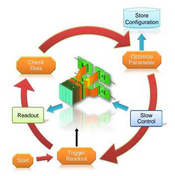
Figure 10.4.: **Concept of the pixel parameter trimming.** An improved pixel configuration is iteratively determined from the digital output of the detector until the trimming goal is achieved.
