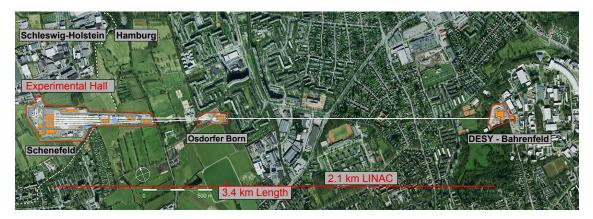
Figure 3.1.: Layout of the EuXFEL in Hamburg [8]. The machine is built in a 3.4 km long tunnel below Hamburg from DESY to the experimental hall in Schenefeld. Most of the tunnel is filled with the 2.1 km long superconducting LINAC, which accelerates the electron beam to 17.5 GeV. In Osdorfer Born, the beam is distributed and transported to the undulators, in which the X-ray radiation is generated. Finally, the X-rays are transferred to the beamlines in the experimental hall.
