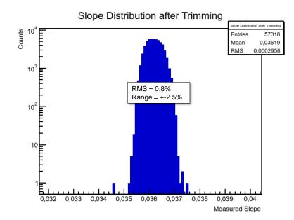
Figure 10.7.: ADC gain distribution after trimming. Target slope was 0.0362. Two full ASICs and some pixels have been switched off during trimming. 99.99% of trimmed pixels end in the expected 2% range.
