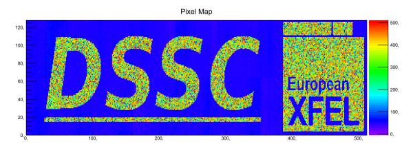
Figure 12.1.: DSSC Logo, generated by a special configuration of the pixel registers. Due to a special configuration of the power-down bit in the pixel registers, the DSSC logo has been generated. This image shows, that the pixel configuration is correctly assigned to the configuration stream and also that the pixel data is correctly received from the PPT and correctly sorted by the software.
