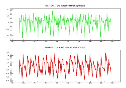
Figure E.3.: Upper graph: DNL. Lower graph: INL. The plot shows a very uniform ADC measurement with a DNL\_RMS of below 5% and an INL\_RMS of round 2%.
