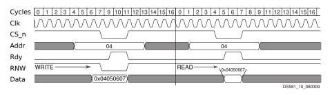
Figure 6.3.: EPC write and read cycles[89].
