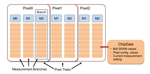
Figure E.2.: Scheme of the root file storage structure. All measurements of the same pixel are stored in the same root tree as separate branch. The branch elements store all data for all iterations and settings linearly in the branch.
