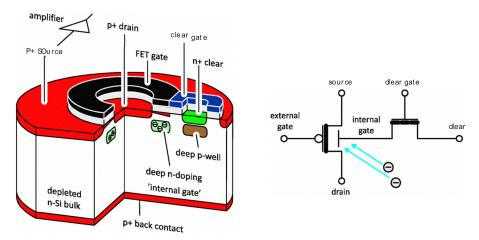
Figure 5.4.: Schema of a DEPFET pixel and the according schematic drawing [78]. Below the outer gate, a deep n-doping implements a potential minimum for electrons that attracts negative charge carriers. Due to the changed potential, positive charge carriers are attracted below the external gate forming a conducting channel. In this way the deep n-doping works like an internal gate. The clear contact is used to remove the trapped charge carriers from the internal gate.
