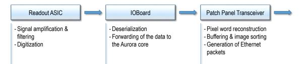
Figure 7.1.: Scheme of the readout chain of the DSSC detector. It is implemented in three hardware levels. The major tasks of the modules are summarized.
