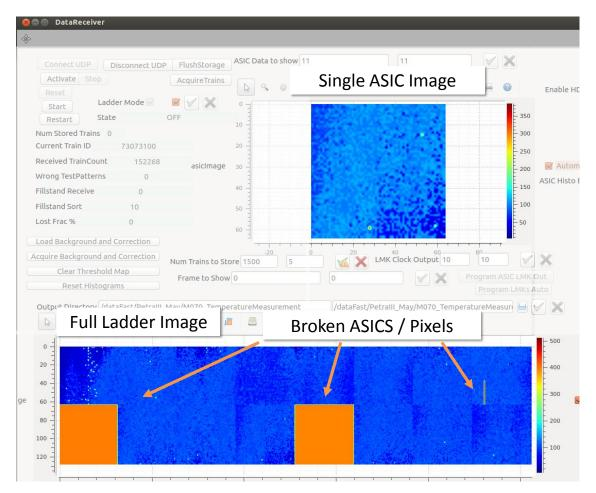
Figure 11.4.: Section of the Karabo Data Receiver Scene. Two Karabo visualization Widgets are shown: the full Ladder image and the single ASIC image. Received image data is directly displayed in the scene.
