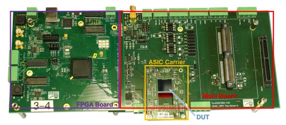
Figure 5.13.: **Image of the ASIC Test System.** The modular setup is composed of three boards. The ASIC Carrier board allows easy change of the DUT, which is glued and bonded on the carrier board. In this way, the setup can also be used for various ASIC generations.
