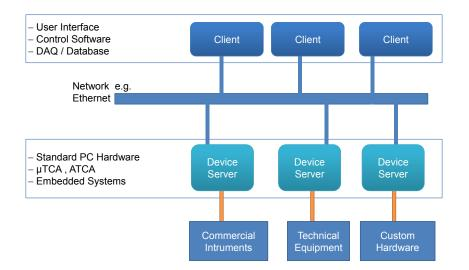
Figure 4.6.: Typical setup of a SCADA system. A central network connects device servers and client applications. The device server is a specialized application that provides distant access to the hardware components. The device server can run on any hardware, in large experiments often  $\mu$ TCA or ATCA systems are used, also embedded systems or standard PCs are possible.
