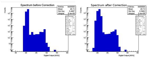
Figure E.6.: Effect of the SRAM correction. The systematic effect has only been max 0.9 bins. But the effect is clearly shown by the much more uniform shape of the spectrum, after correction on the right side.
