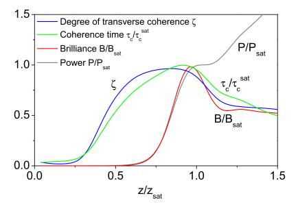
Figure 2.6.: Schematic overview about the FEL properties along the undulator [10]. An FEL reaches the highest performance when the micro bunches can not be further compressed. The first saturation of an FEL in the soft X-ray region was reached in 2003 at the TESLA facility in Hamburg, Germany [11].
