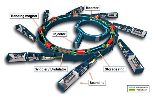
Figure 2.2.: Schematic setup of a 3rd generation light source synchrotron. Several beamlines, which contain the different experiments, are attached to the central electron storage ring. The electromagnetic radiation is generated in the bending magnets, wigglers or undulators [3].
