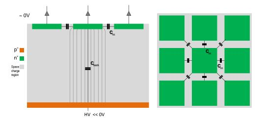
Figure 5.2.: Schema of a pixelated n<sup>+</sup>-in-n diode array [73]. The input capacitance mainly couples against the neighboring pixels. For good charge collection capabilities the anode needs to fill large area of the pixel.
