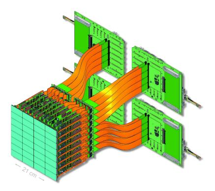
Figure 1.1.: Artistic image of the DSSC megapixel detector. (Courtesy of K. Hansen, DESY)
