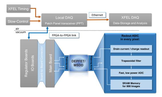
Figure 5.1.: Block diagram of the DSSC detector [68]. For each sensor pixel, one readout channel is implemented in the ASIC, which is bump-bonded on the backside of the sensor. The sensor routes the ASIC signals via wire bonding to the Mainboard. Several PCBs implement the infrastructure for readout, control and power distribution.
