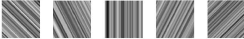
Figure 4.5: Synthetic EPIs for disparity values of -1, -0.5, 0, 0.5, 1 pixel (from left to right).
