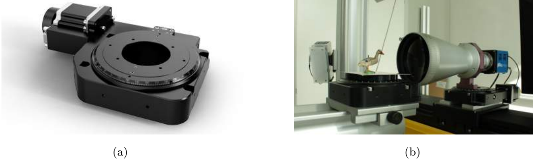
Figure 5.13: Circular light fields acquisition setup: the rotation stage OWIS DTM 130N (a), and the whole setup with the telecentric lens Zeiss Visionmes 105/11 (b).
