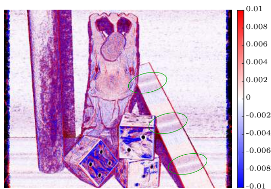
Figure 4.18: Disparity errors of the structure tensor for a disparity range of 4px and three refocusing steps. To compute the difference, both estimated disparity and ground truth have been scaled to fit a 2px disparity range, and thus the error also refers to this range; this allows direct comparison with Figure 4.16 (e). To highlight the behavior of the estimates around the refocused disparities (9, 10 and 11) we clipped the errors to \pm 0.01px and added three green circles.
