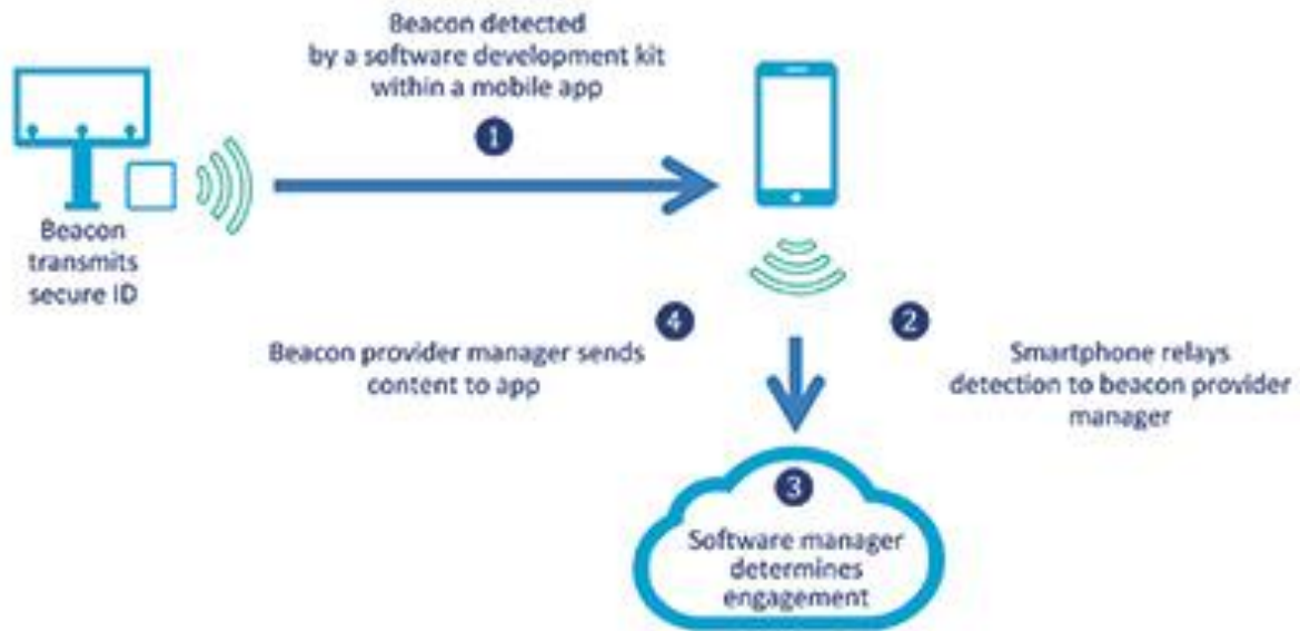
Figure 2.8: How Bacons Work (Adapted from infodisplay 2015)
