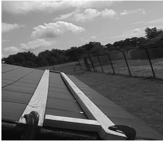
Figure 13 Shading 3a-Si with battens
