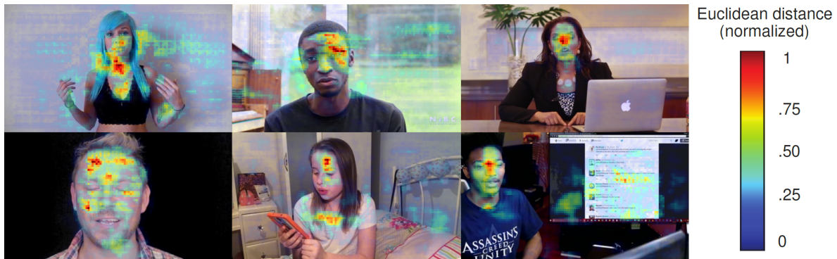
Figure 4. Visual pixel-level occlusion analysis. Each image shows the changes in trait predictions as a function of location resulting from systematically masking a representative example input overlaid on the input itself. Masks are defined as 10 \times 10 pixels centered on every fourth point in the spatial axes. Change is defined as the Euclidean distance between the predictions before and after masking the inputs.
