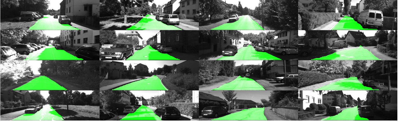
Fig. 2. Examples of road detection results by our stereo-based vanishing point constrained Dijkstra road model.
