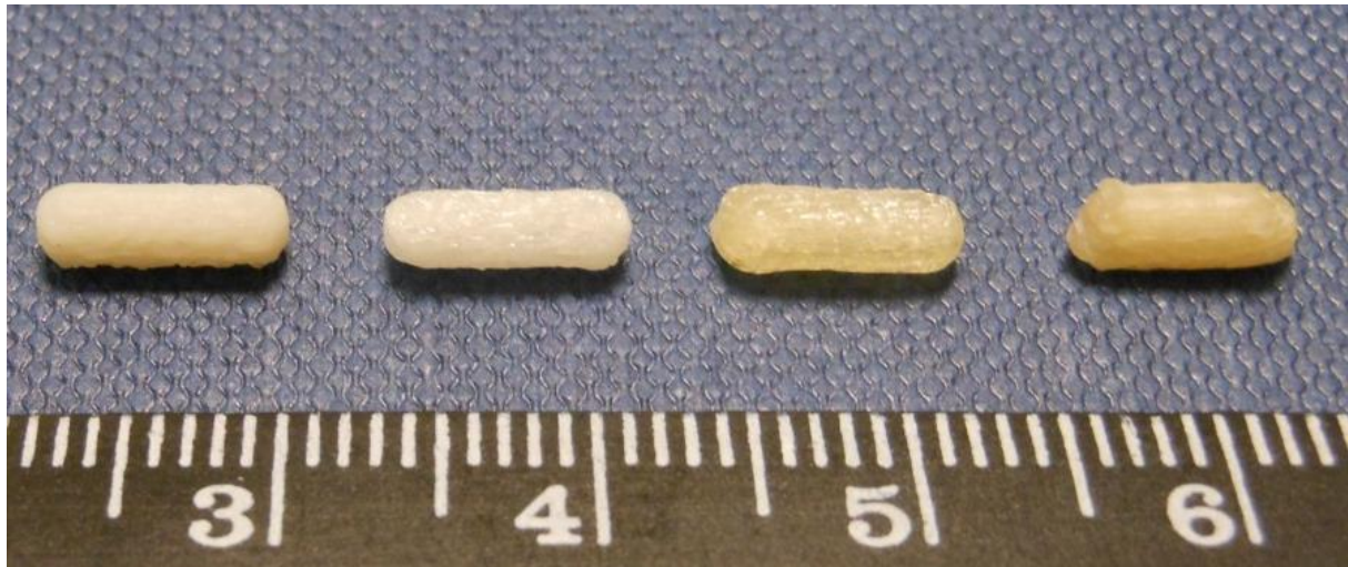
Figure 2. From left to right pictures of 3D printed devices of Kollicoat IR, Klucel EF, Aqualon N7 and Aquasolve-LG (units are cm).
