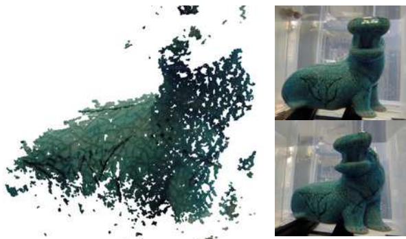
Figure 11. Close look at the underwater 3D reconstruction of a statuette using the proposed RSfM approach.
