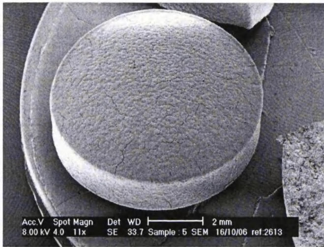
Figure 5.13a Surface SEM of Eudragit S coated prednisolone tablet (no plasticizer).
