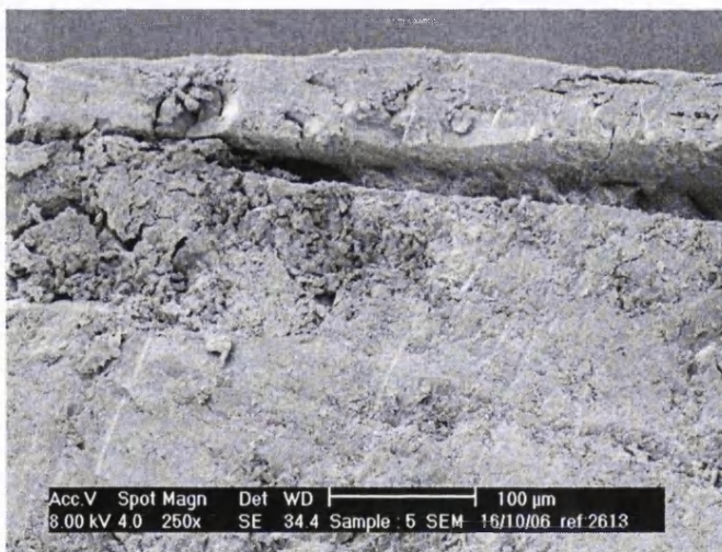
Figure 5.13b SEM cross-section of Eudragit coated prednisolone tablet (no plasticizer)
