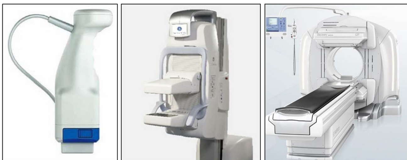
Fig. 2 Range of CZT imaging devices: CZT has been used in a range of devices including small hand-held imaging probes for intrasurgical use (crystal photonics) (left), small planar detectors used for breast
