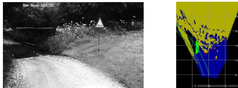
Figure 7.24. Detected ford corresponding to location 1. On the right – crest/ditch map where green colour corresponds to identified objects
