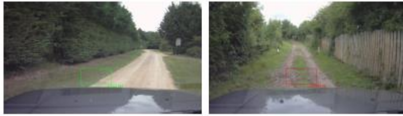
Figure 6.17. Examples of mixed surface samples: left – transition between gravel and grass, right – track with grass patch in the middle.
