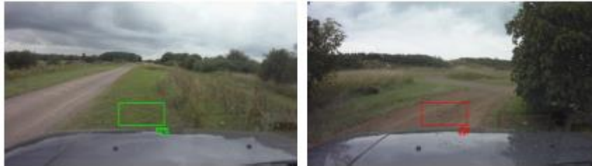
Figure 6.2. Example images of the classified samples. Only the area highlighted by the colour rectangle is used as an input of the classification algorithm. The colour of the bounding box signifies the result of the classification process: green - grass (left), red non-grass surface (right).
