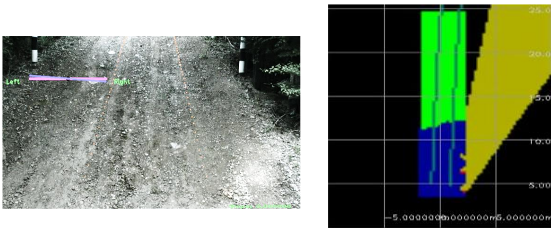
Figure 7.10. Illustration of steep slope in front of the vehicle covering entire field of view.
