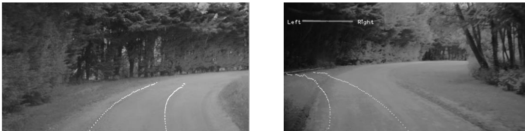
Figure 8.20. Surface profile measurements are based on the predicted vehicle path taking into account the driver steering inputs (measurement points are denoted as white dots).
