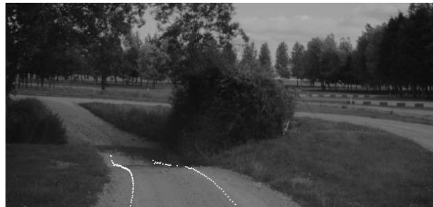
Figure 8.18. Ford in the developing world track. White points depict the predicted vehicle path.
