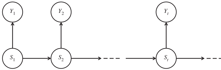
Figure 2. Directed acyclic graph of a hidden Markov model where S_t is the unobservable states and Y_t represents the observable time series.
