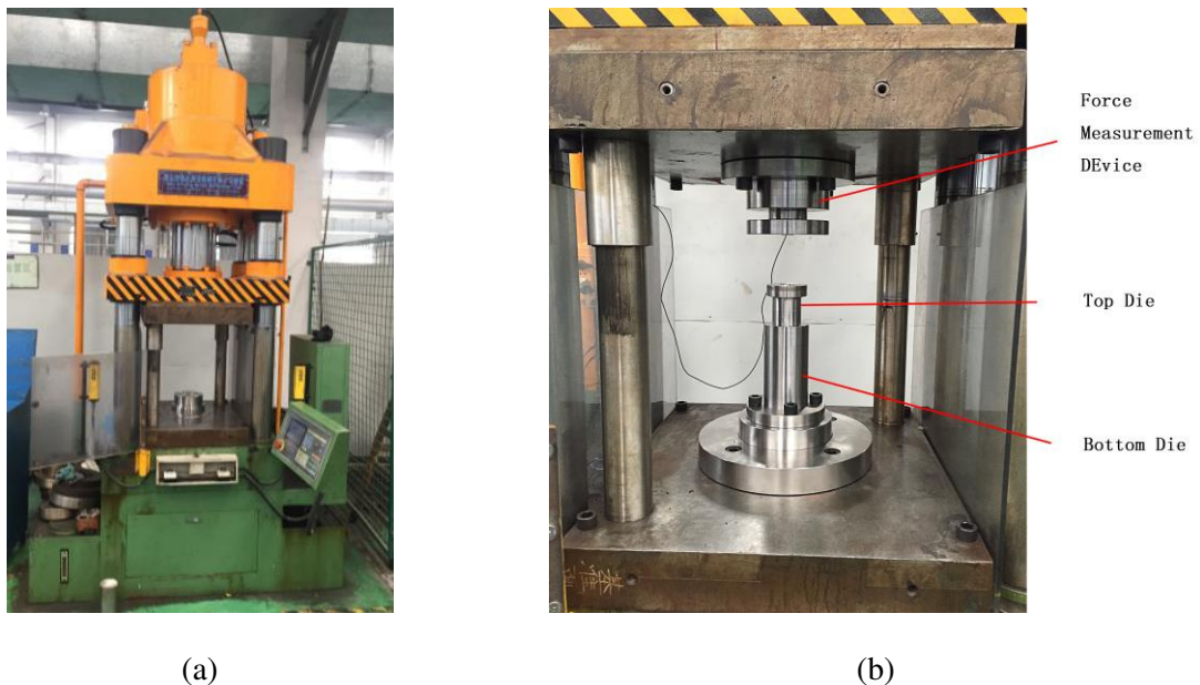
Fig. 8: Forming press and tools, (a) 3000 kN vertical hydraulic press, (b) the experimental setup.
