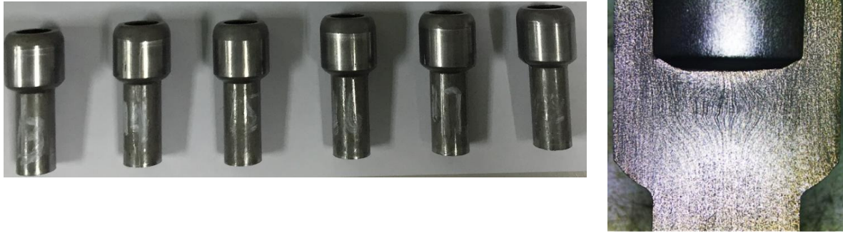
Fig. 22: Sample parts formed and grain flow line of a part under a microscope
