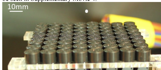
Fig. 14. An 8x8 array trapping an Expanded Polystyrene Particle 20 mm above the array.
