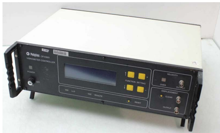
Figure 5.8: Polytec OFV 3001 vibrometer controller for higher accuracy measurement
