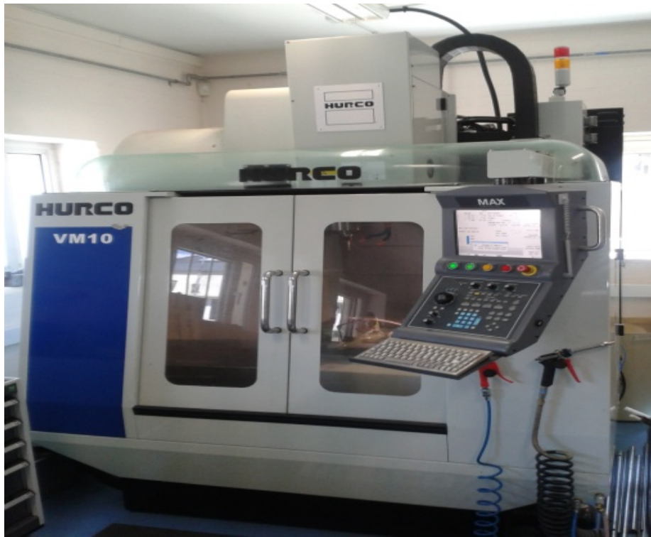
Figure 4.12(a): The HURCO VM 10 CNC machining centre
