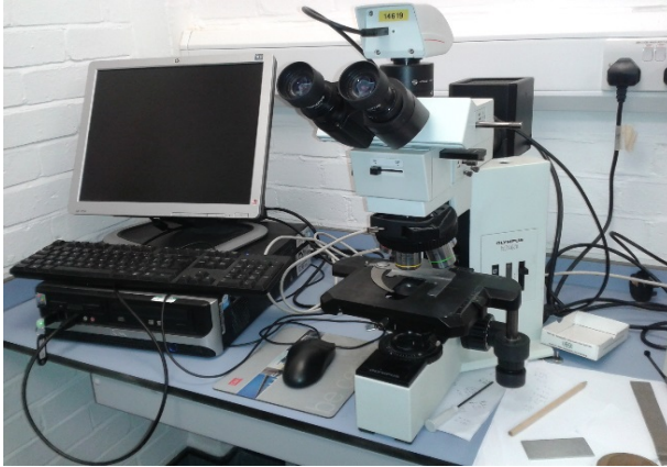
Figure 5.2(a): A typical OLYMPUS BX 40 computerised optical microscope
