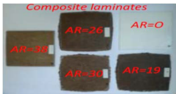
(b) HFRP/PCL composite laminate specimens
