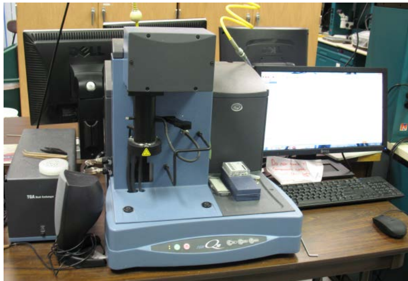
Figure 4.5: A Q50 V 6.1 Thermogravimetric analyser
