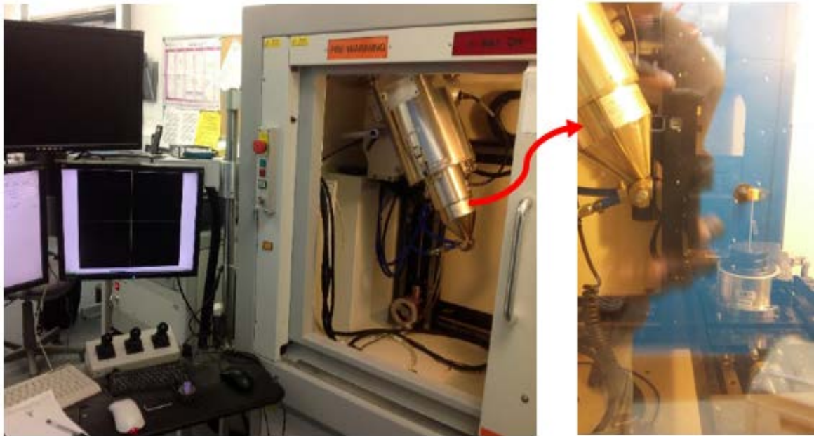
Figure 5.3(b): Scanning FRP specimen with Metric XT H 225 Microfocus X-ray micro CT Scanner
