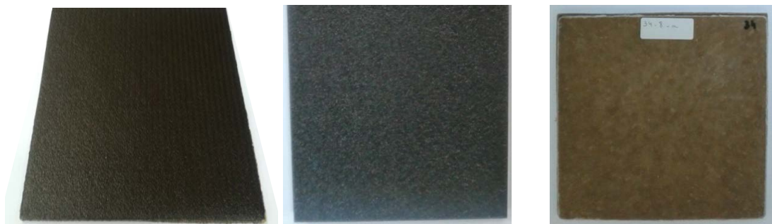
(a) MTM 44-1 CFRP/EP laminate.
