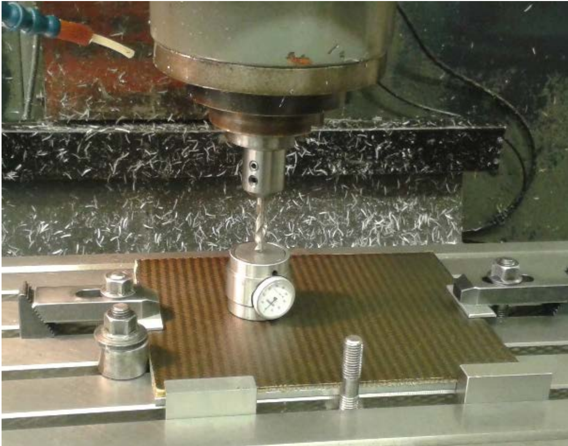
Figure 4.10: Calibration and gauging of the drilling set-up
