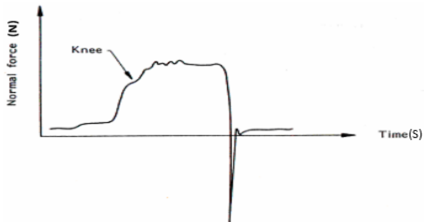
Figure 3.10: Typical axial force history during composite drilling (Abrate & Walton, 1992)
