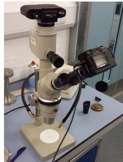
Figure 5.2(b): Set up showing measurement of delamination zone
