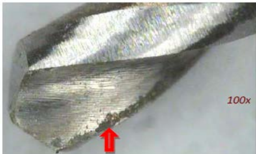
Figure 3.5: Twist drill edge chipping type of wear at lip (Rahman et al., 2009)
