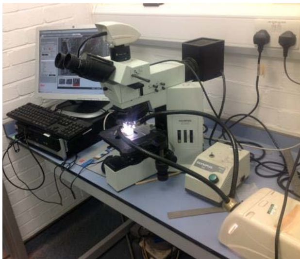
Figure 5.2(b): Set up showing measurement of delamination zone
