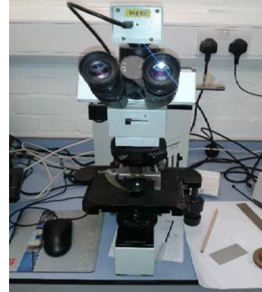
Figure 5.2(a): A typical OLYMPUS BX 40 computerised optical microscope
